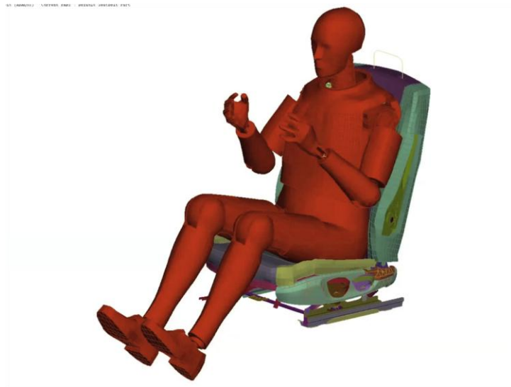
Figure 1. Combined dummy seat model
